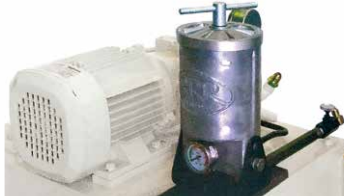
Hydraulic oil filtration equipment
